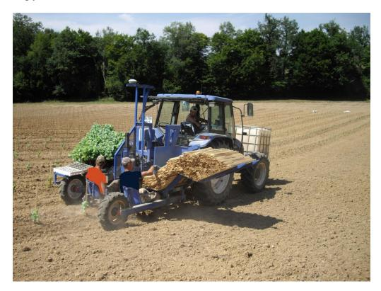
The machine opens a furrow 30cm deep, plants the stake, positions the young plant after the stake, and the earth begins to cover the plant. The machine waters it and finally the furrow is closed by two parts mounted on a parallelogram. The functions are controlled by the robot, which gives precise points to plant the stake, positioning the young plant and watering it. It aligns the plants on the line and its perpendicular and it determines the distance between ranks.
